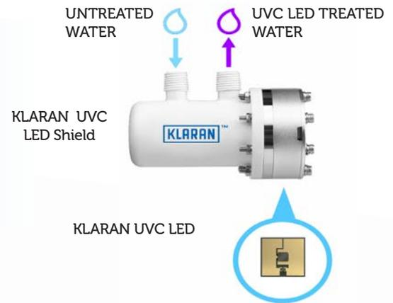
The Klaran Shield consists of small chamber through which the water flows from the Direct Chill Tank to the Tap. On its way the water is exposed with UVC LED wavelength radiation which is highly effective in destroying water-borne Bacteria and Viruses
