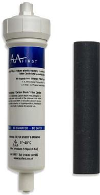
A Carbon Block Filter is the standard Filter used for Water Coolers. Its Filter housing should be made of food grade material and the Carbon Block should be of a pore size to remove 95% of solids above 1 micron to create a barrier against Giardia, Cryptosporidium and Cysts.
